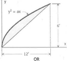
Find the moment of inertia about the indicated x-axis for the shaded Q.5(B) area shown in Figure.
